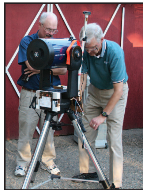
Greg Johnson looks on as Walt Morgan sets up to observe lunar occultations. Walt's system includes a GPS receiver, a "Kiwi box" time stamp inserter, and a camcorder as well as an 8-inch Meade LX-200 telescope.
