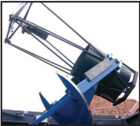
Cindy Foote's 16-inch telescope at Vermillion Cliffs Observatory. Her CCD camera is mounted at prime focus. The telescope's truss is made of carbon fiber tubes.
