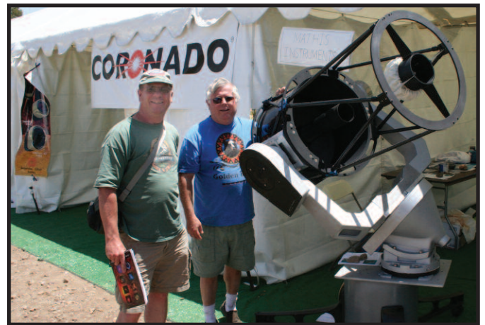
Workshop participant Tom Smith stands beside Tom Mathis and the Plane Wave Instruments 20-inch optical assembly on a Mathis fork mount. Dave Rowe gave a talk at the workshop on his development of the corrected Dall Kirkham (CDK) optics. Photo taken by Russ Genet at RTMC a few weeks before the workshop.
