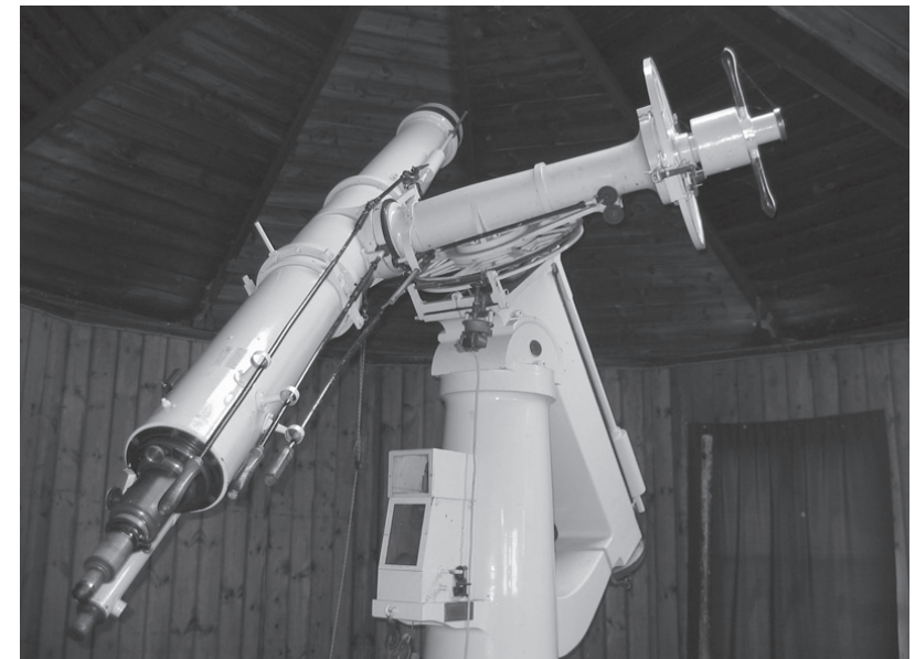
Figure 1: 8-inch Cooke refractor used by the author for double star measurements.
