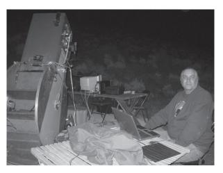
Figure 8: Dan Gray and his 14-inch alt-az robotic telescope, affectionately called "Lollipop" (for obvious reasons). Dan was working to fully automate near infrared aperture photometry.
