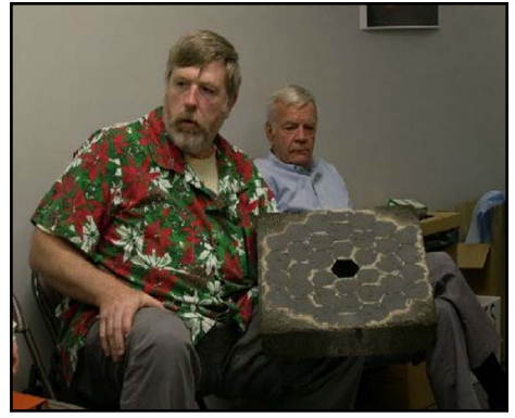
Left, Thin 3/4" - 75 lb mirror from DOTI Center: Joe Haberman testing the 1 meter meniscus mirror from DOTI Right: David Davis with first attempt at Foamglas tessellation
