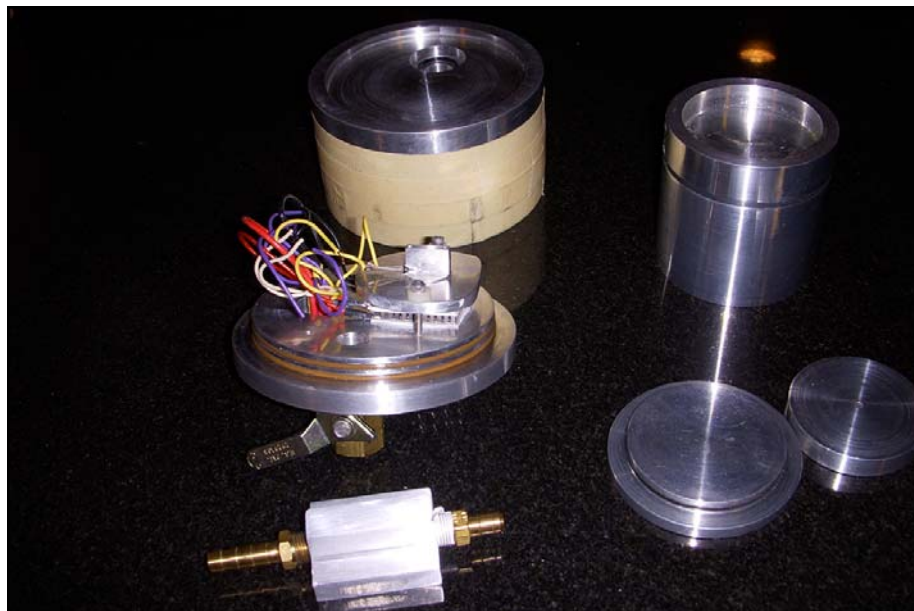
Machined parts for the Jones near IR photodiode photometer. The vacuum cryostat allows low temperatures to be maintained with a multistage thermoelectric cooler, thus reducing detector noise, the major noise source for photometry in the J and H bands.
