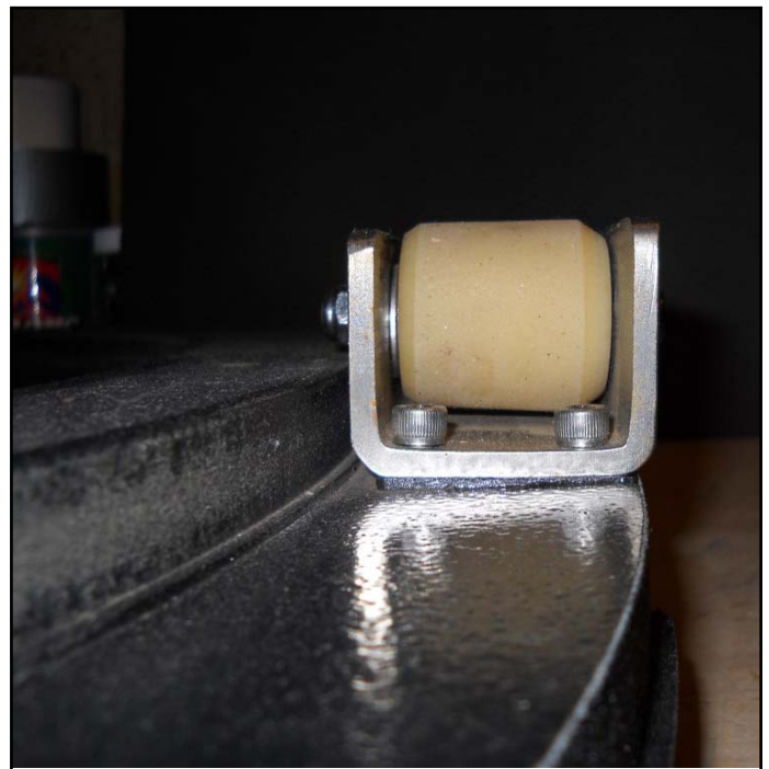
Below: Illustration of conical wheels. Top shows an exaggerated design of a conical wheel to better illustrate the principle and the lower shows an example of a “crowned” conical wheel. Right: Photo of conical wheel from drive on Howard Banich 30” scope.
