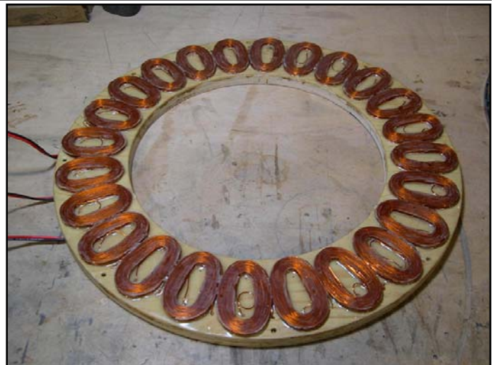
Direct Drive motor prototype, which consists of coils and permanent magnets set up on opposing rings.
