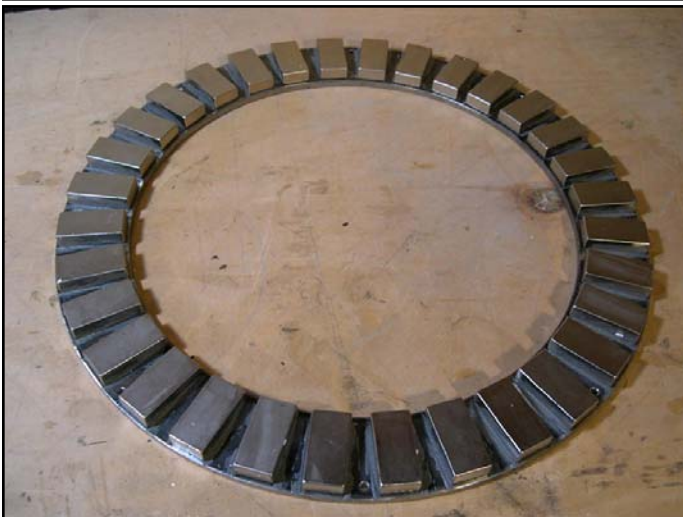
Direct Drive motor prototype, which consists of coils and permanent magnets set up on opposing rings.
