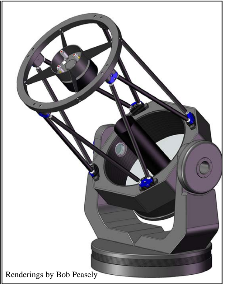
Two views of our 0.7-meter alt-az conceptual design. The combination of an alt-az mount, lightweight structure, and dual Nasmyth foci could provide a compact, portable, low cost, easy to use, research-grade telescope.
