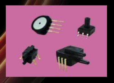
Precision capacitance based sensors for ~\$200
