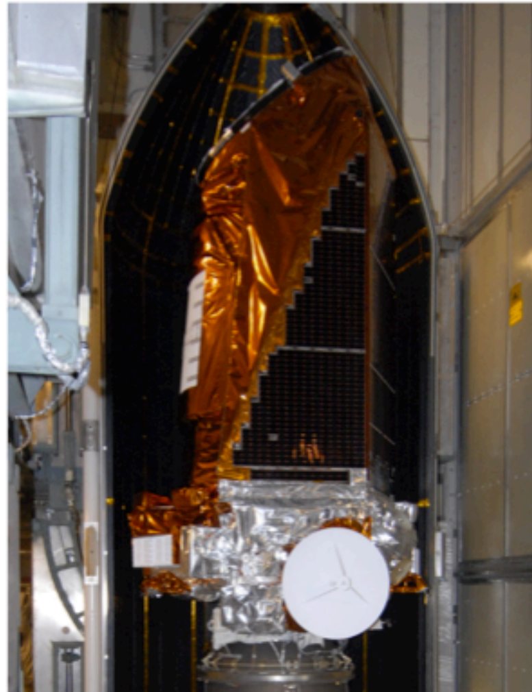
Fully assembled Kepler photometer Mounted on the spacecraft
