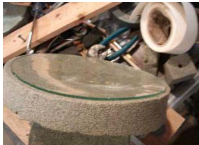
Reflections show a potato chip surface to the blank. Notice the reflection of the board on the left and the 'puddle' reflection of the paper roll on the right. This was an excellent fusion but the final curve made the puck unusable.
