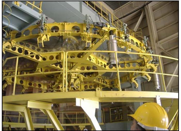
When the thin meniscus mirror is removed from the telescope and brought down to be recoated, it must be very carefully supported in this mirror transporter.
