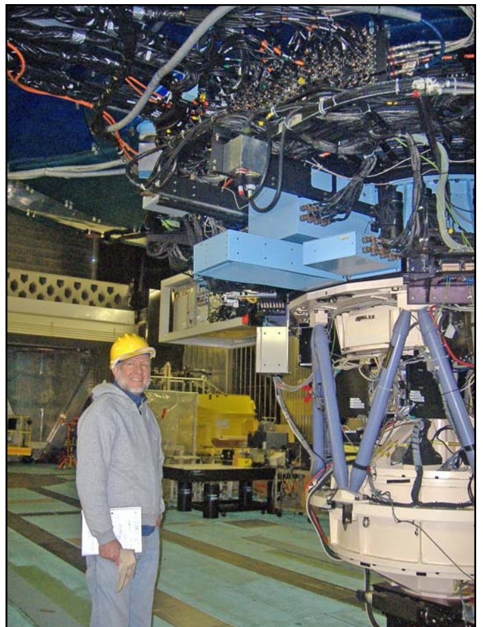
Below: Russ stands under the Subaru telescope beside the Cassegrain focus instruments. This is just one of the four focus positions.
