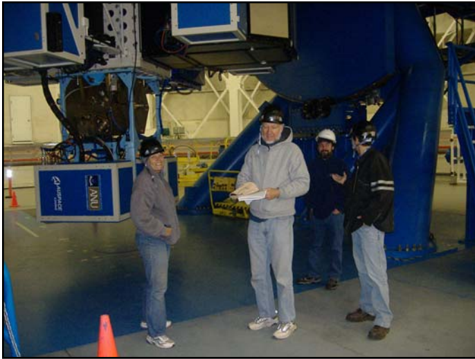
Cheryl, Russ, Chris and Jon stand by Gemini's Cassegrain focus. One optical path is straight through to the bottom instrument behind Cheryl, while four other instruments are above
