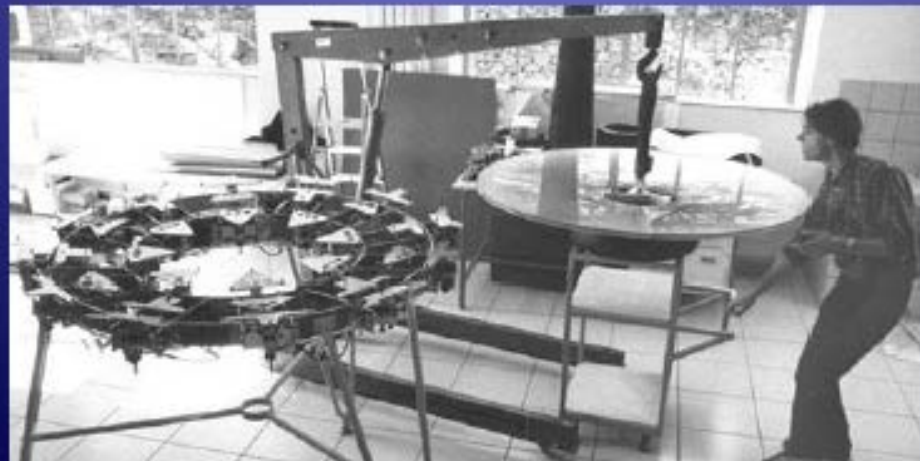
French ATM with 1-m meniscus mirror and astatic support system
