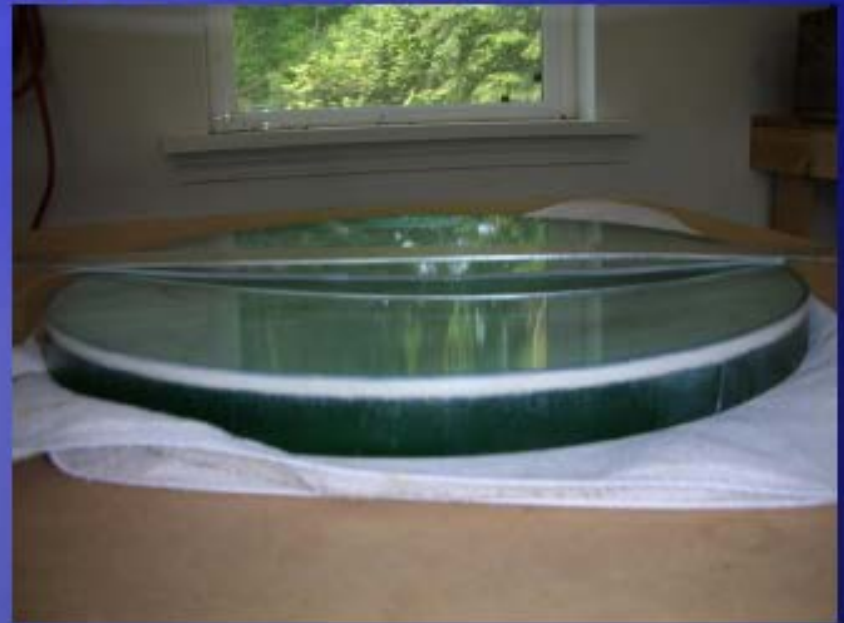
Mel Bartle's 13" soda lime slumped meniscus mirror
