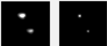
Figure 3: Left is the first 500 images just stacked. Right is the best 10% of the first 500 images (i.e. 50 images) stacked and aligned.
